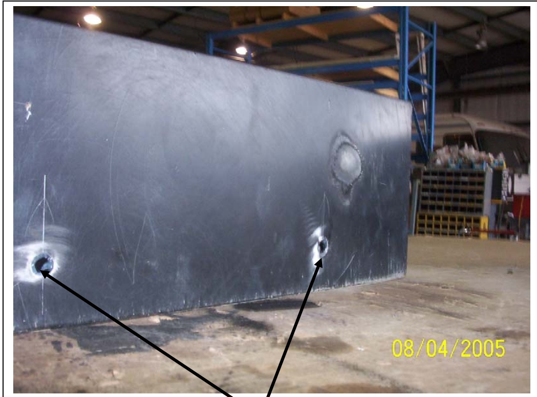
Drain holes drilled in evaporator box using the drain pan supplied as a pattern. Ensure holes line up with the holes in the body of the machine for drainage.
