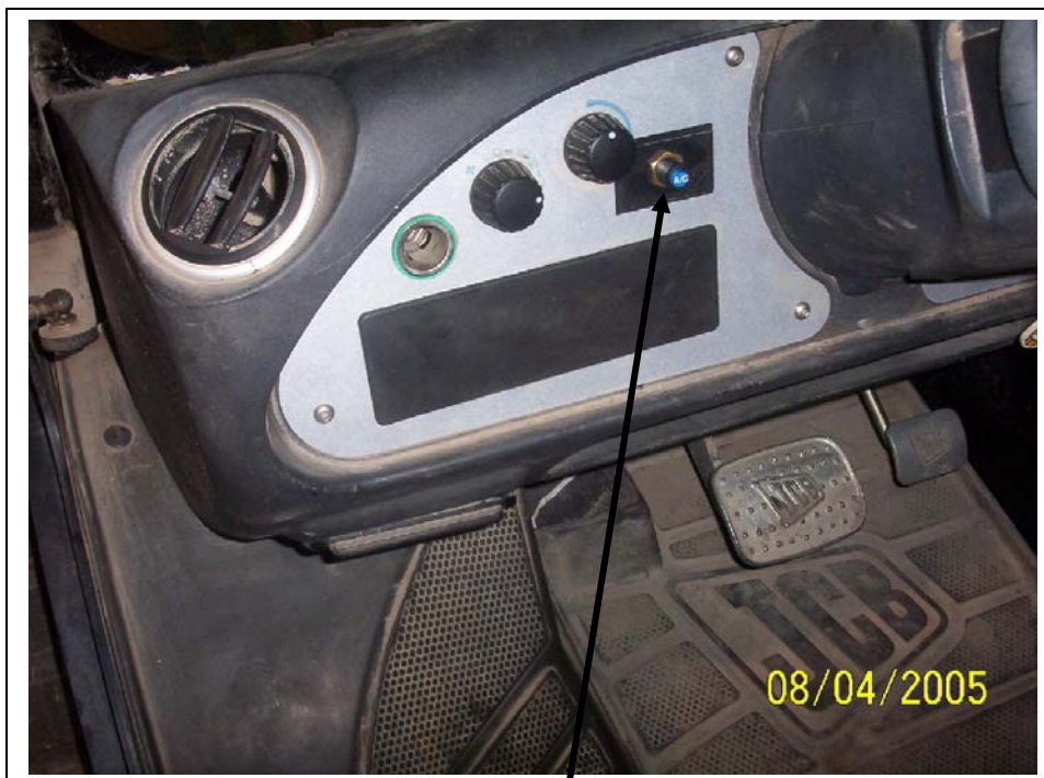
A/C switch installed.
